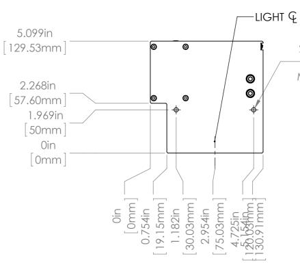
2X Ø 0.197in[5mm] THRU ALL M6X1.0 - 6H THRU ALL MOUNTING HOLES-BOTH ENDS
