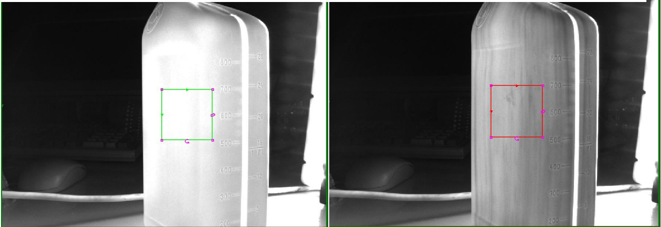
Above: Left - Raw image of a good bottle. Right - Raw image of a streaked bottle. Below: Filtered images of the bottles above.
