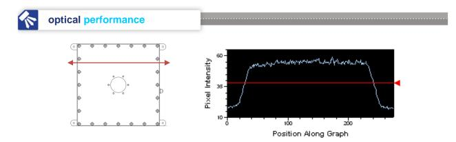
The DLPW Washdown offers a very diffuse light pattern at any defined working distance. The Pixel Graph representation shows a steep drop off in intensity outside of the active area with a very diffuse light pattern inside.
