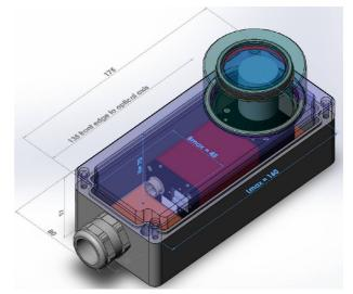
Chameleon ST, 80x92x175 (w x h x l) for angular **C-mount cameras up to 45x70x160mm** (w x hx l including connectors).
